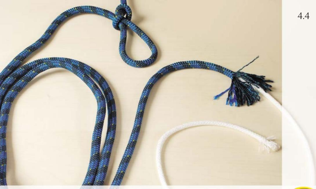
Pull out a length of core x 80 the diameter of the rope. This only applies to products with an inner middle cover.
