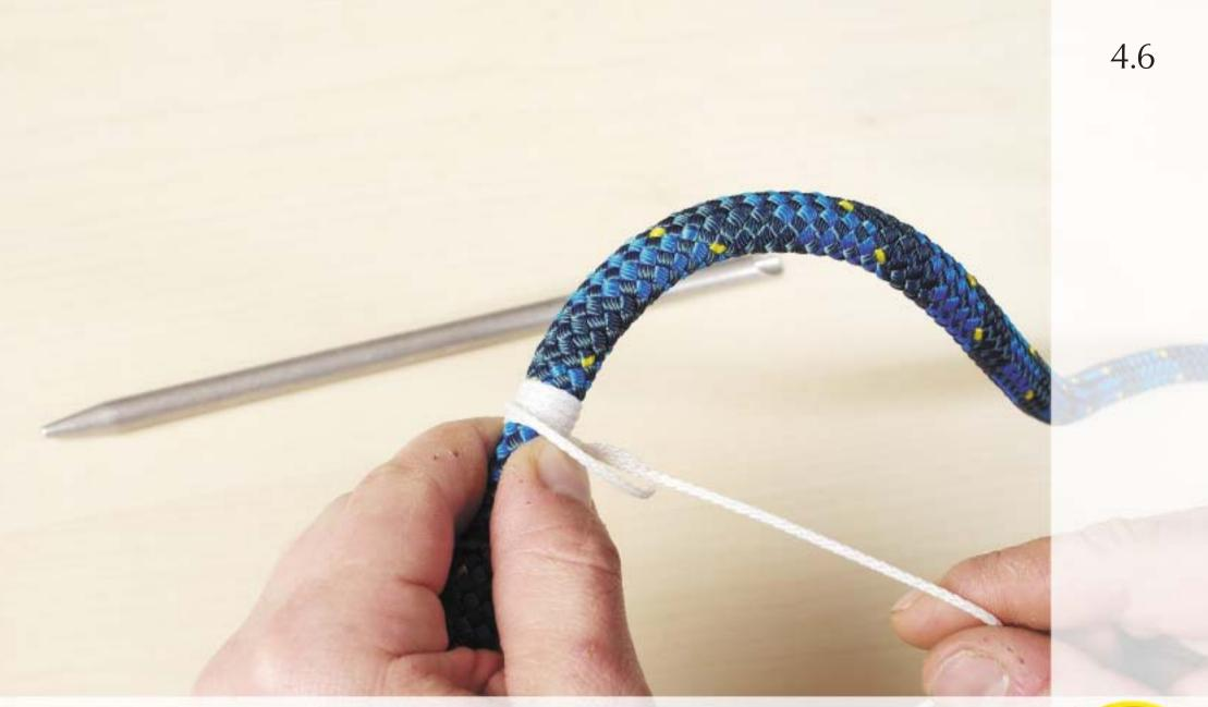
Make a 1 cm wide whipping 40x the diameter of the rope from the end of the splice.
