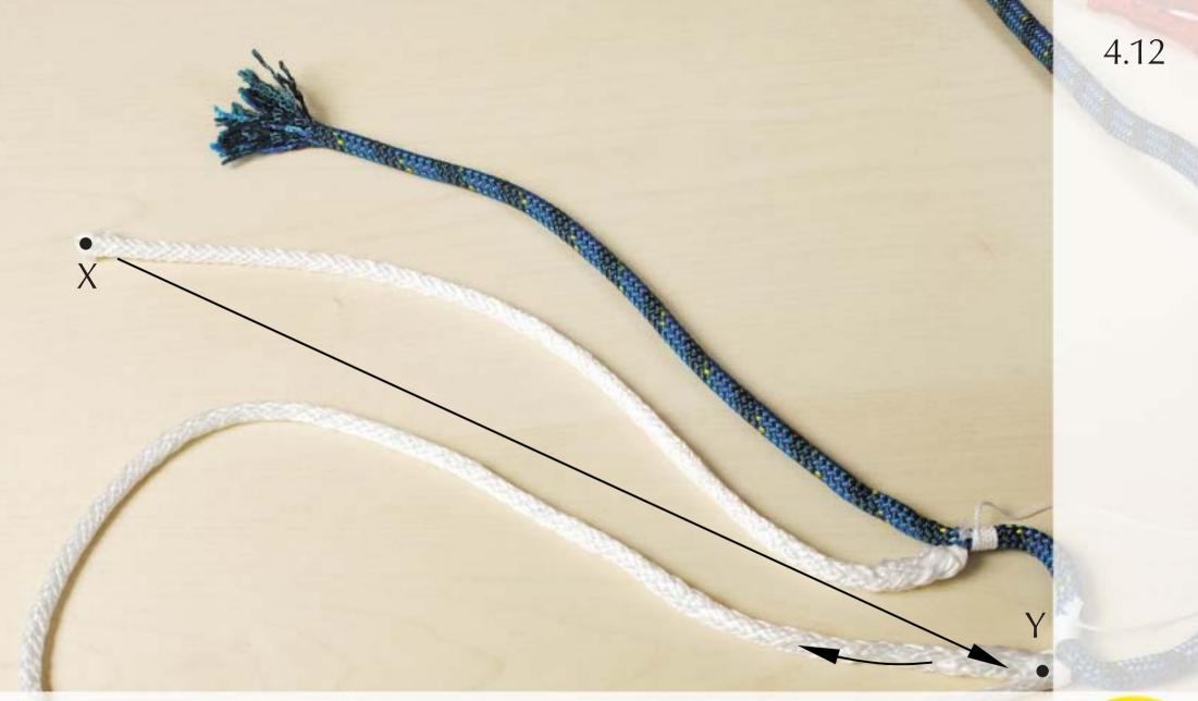
Insert the core marked X into the core marked Y using the specialised fid.
