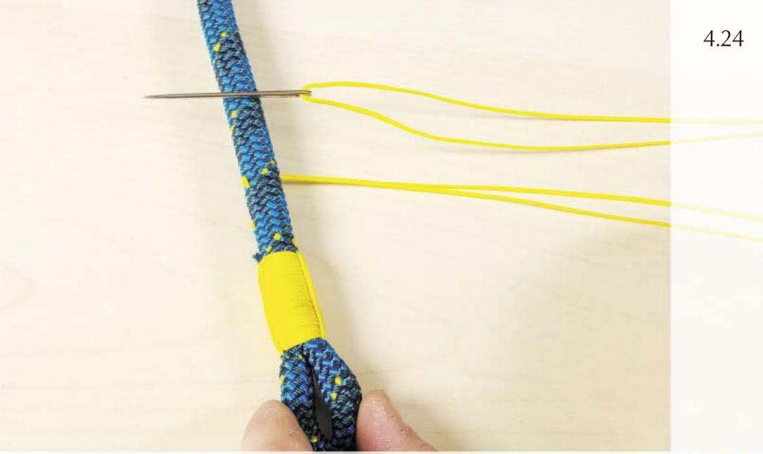
After the 4 cm whipping is completed anchor the twine by sewing backwards and forward through the rope several times.
