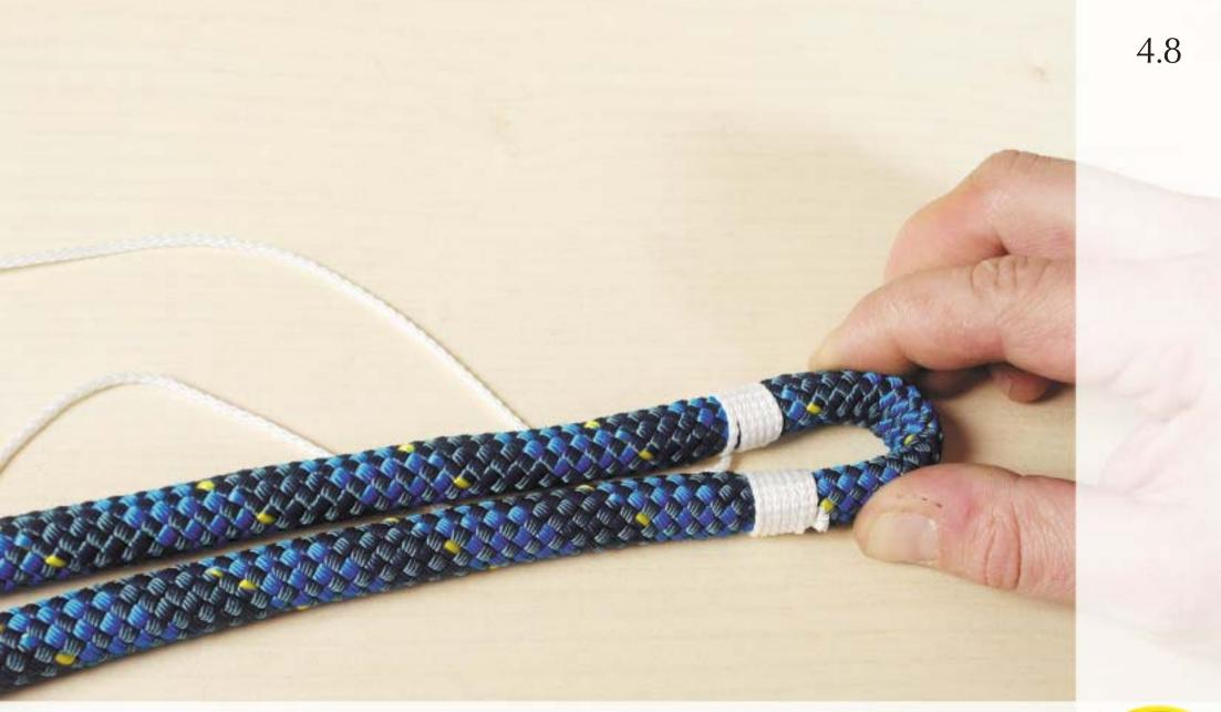
When inserting a thimble line up the two whippings with bottom open end of the thimble.
