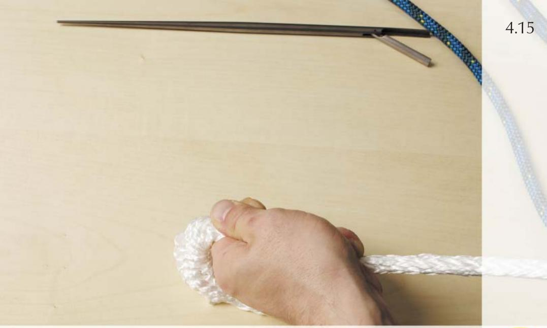
Milk down the outer core over the inner core until it has completely disappeared.
