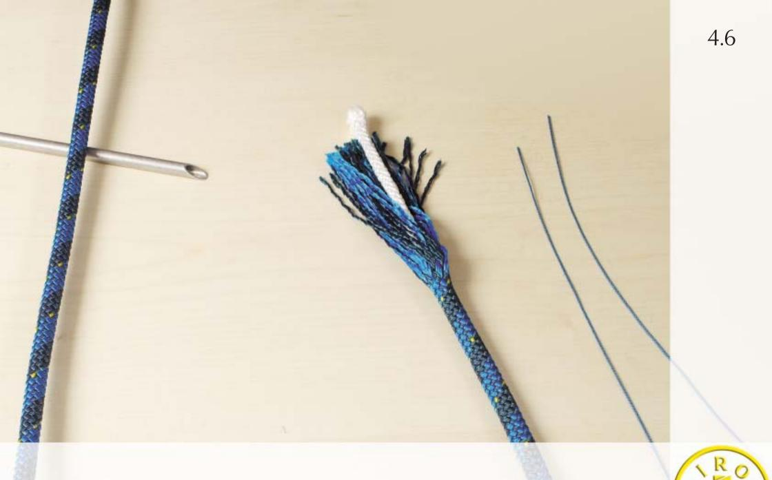
Slide the cover back until it is level with the inner core.
