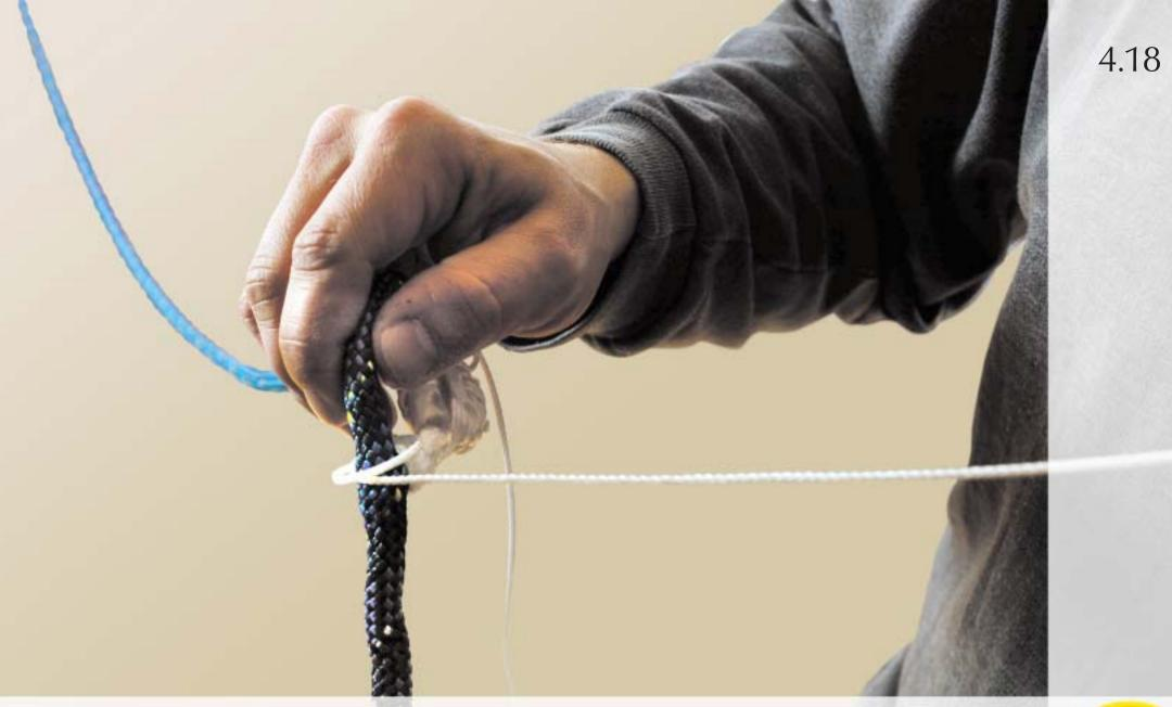
Remove the whipping just before the completion of the eye.
