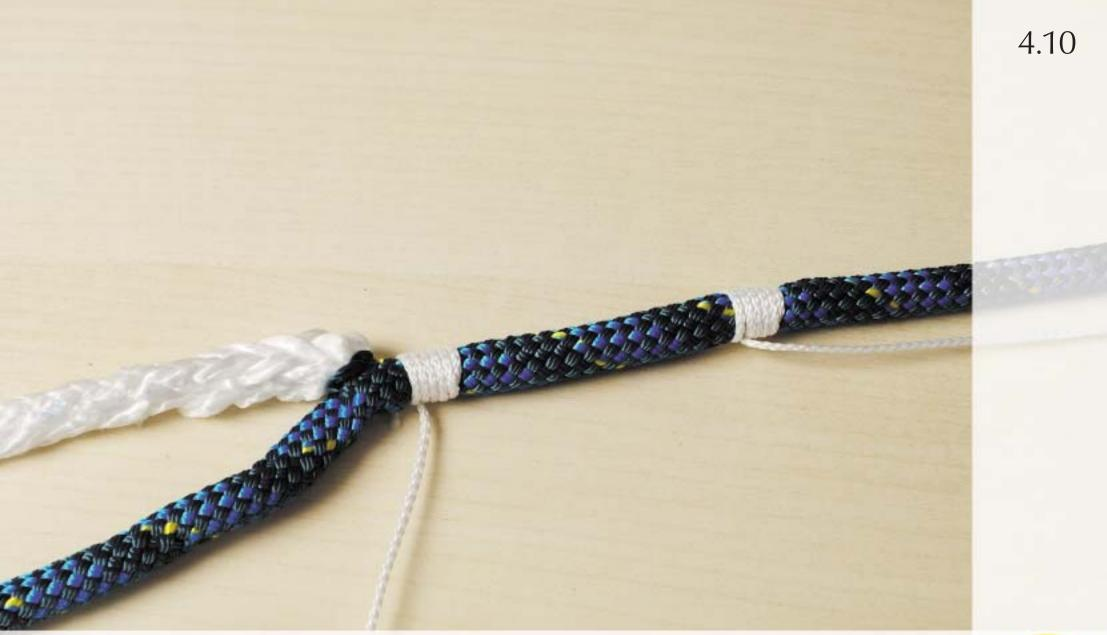
Carefully prise open the outer cover just in front of the first whipping.
