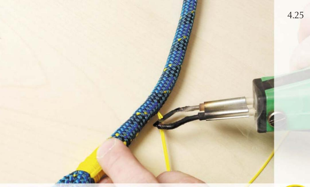
Cut the whipping twine as close as possible to the outer cover and gently press it into the cover.
