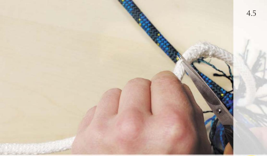
Carefully cut the inner cover and slide it off the core. This only applies to products with an inner middle cover.
