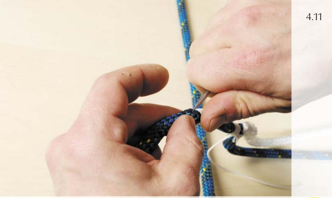
Open up the outer cover after the second whipping and pull out the core. Take care not to damage the whipping pull out the largest possible loop.
