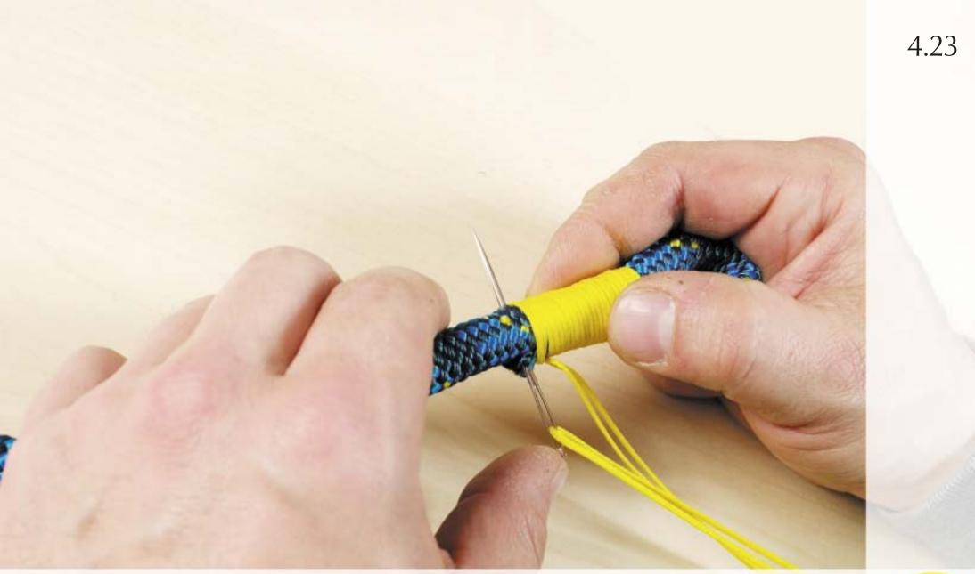
After the 4 cm whipping is completed anchor the twine by sewing backwards and forward through the rope several times.
