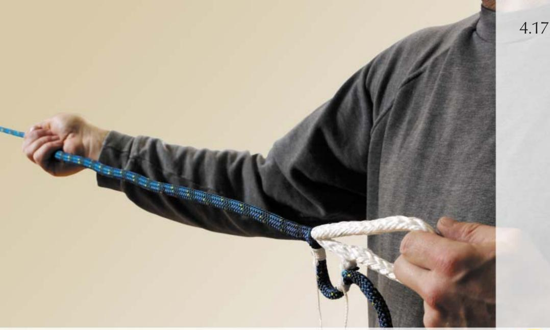
Put the knot made in step 4.1 onto a secure fixing and start to milk down the cover towards this eye.
